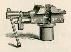
A new and useful vise, for holding all shapes and sizes of articles for drilling in our drilling machines. Has steel jaws; hole through shank to take any length. Arranged so as to be in center with spindle, or, if desired, can be thrown to one side. Jaws are operated by right and left hand screw.
