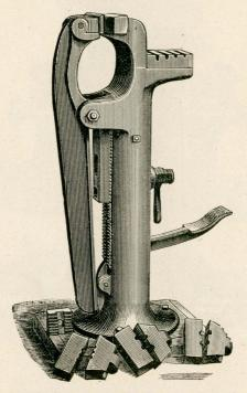
For forming, sharpening, and welding calks on horse and ox shoes, for making bolt heads, and takes the place of an ordinary vise for bending and shaping hot iron, thus combining two machines in one.
